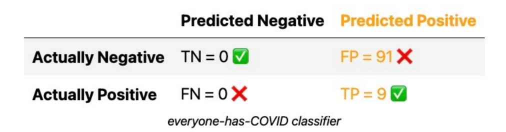
The precision of a binary classifier is the proportion of predicted positive instances that are correctly classified.
